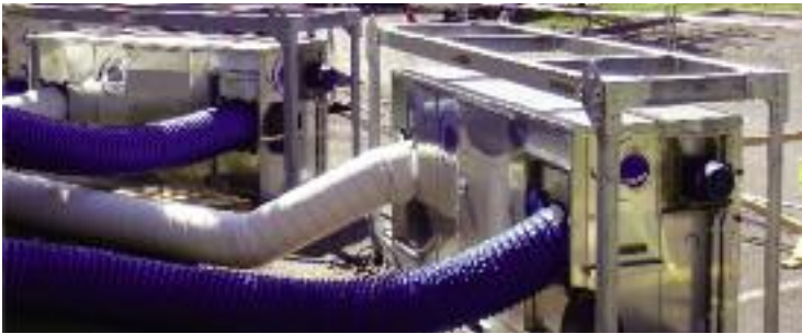
Wet side, MS-6000/5000 pulls moisture from ambient air.
